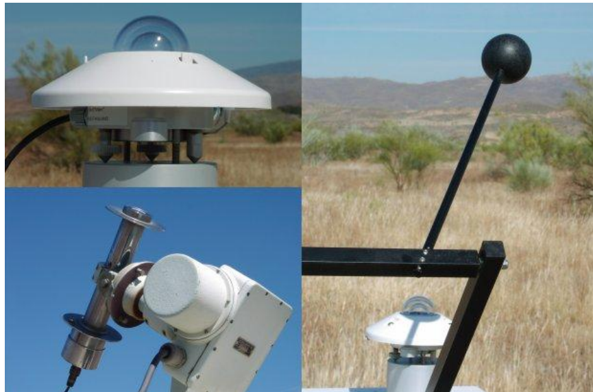
Figure 45: Pyranometer (left top), Two-axis tracked pyrheliometer (left bottom), Pyranometer with shading ball (right) (5)
